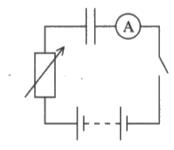
The capacitor is initially uncharged. When the switch is closed, there is a current in the circuit and the capacitor charges.
