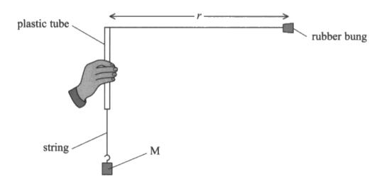
A small movement of the hand causes the rubber bung on the end of the string to move in a circular path of radius r. The rubber bung and the string may be assumed to rotate in a horizontal plane.
